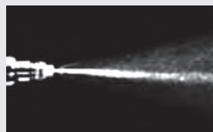
Injector spray pattern before P.i. treatment.
