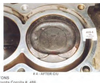
Picture I - Piston after P.i. treatment
